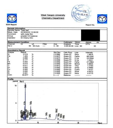
Figure 1 EDXRF spectrum of Teak leaves powder
